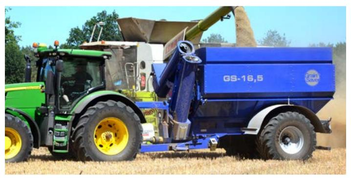
A grain cart, adapted to serve one large combine in operation or two mid-size combines. It requires a 120 hp tractor for smooth operations.
