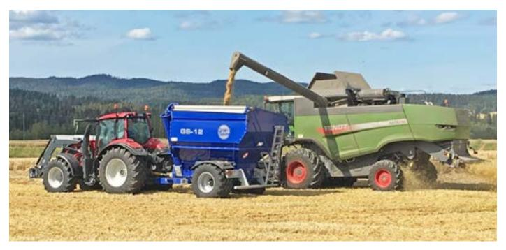
Strong overloading wagon, designed with many years experience from the larger Grain Saver trailers. Perfect for alpine areas, Nordic areas and smaller operations, where efficiency and technical solutions is in focus. Serves easily a mid-size combiner. 80 HP tractor needed.
