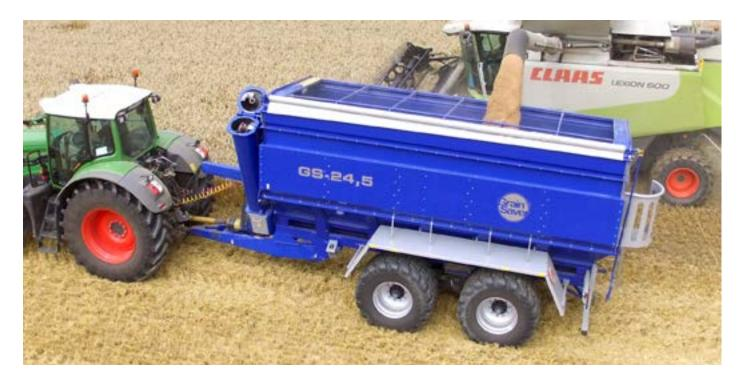
Powerful grain cart, adapted to serve two standard large combines in operation. It is easy to drive. Thanks to its design, it has a large surface area relative to volume. The wagon is equipped with a steerable BPW tandem axle. Unloading time is app. 3 minutes. It requires a 200-250 hp tractor for smooth operations.
