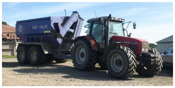
A grain cart developed to serve one large combine in operation or two mid-size combines. Serves easily with a 120 HP tractor.
